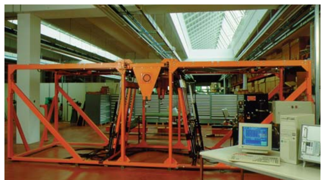
In-house computer controlled dynamic windload simulator.
